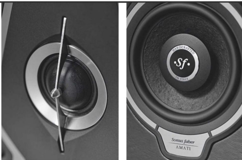
ABOVE: Both the 28mm soft-dome DAD 'Arrow Point' tweeter [left] and new 150mm cellulose fibre midrange driver, with neodymium magnet [right], include proprietary plugs to manage anti-phase behaviour, improving both response extension and off-axis dispersion
